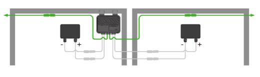
If connecting a TS4-A-2F to only one solar module, connect the TS4 #2 input cables to each other.
