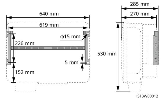
Figure 4-12 Mounting bracket dimensions
