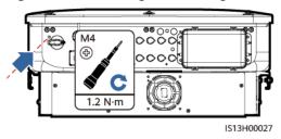
**Step 5** Turn off the DC switch (if any) between the SUN2000 and PV strings.
