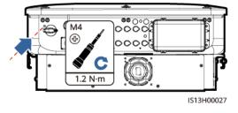
**Step 2** Install the SUN2000 onto the mounting bracket.
