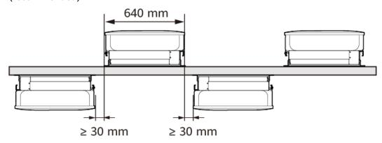
**Figure 4-9** Support-mounted dual-track back-to-back installation (not recommended)
