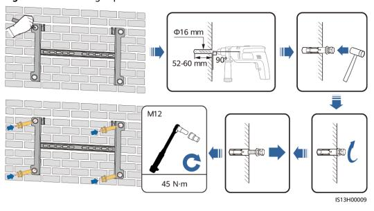
Figure 4-15 Installing expansion bolts
