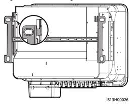
**Step 3** Tighten the nuts on both sides of the SUN2000.
