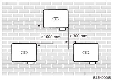
Figure 4-5 Three-layer triangle installation (not recommended)
