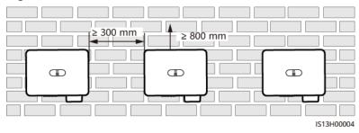
Figure 4-4 Two-layer triangle installation (not recommended)
