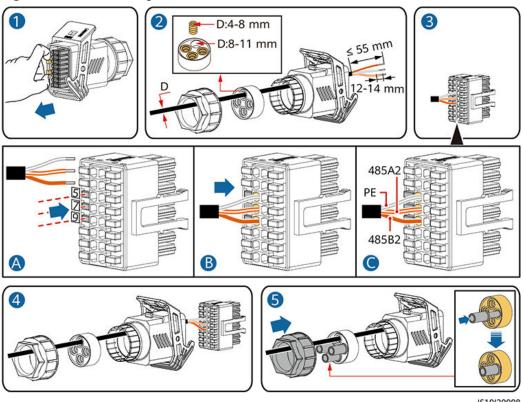
Figure 5-26 Connecting the cable
