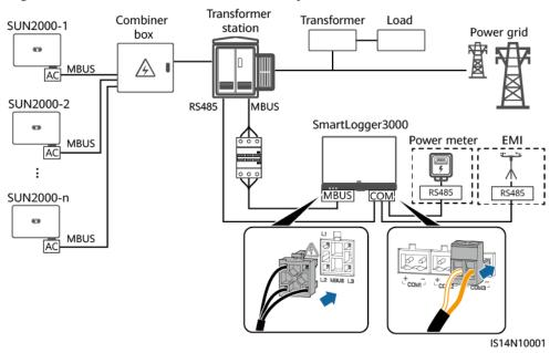
Figure 5-22 MBUS communication (utility-scale scenarios)
