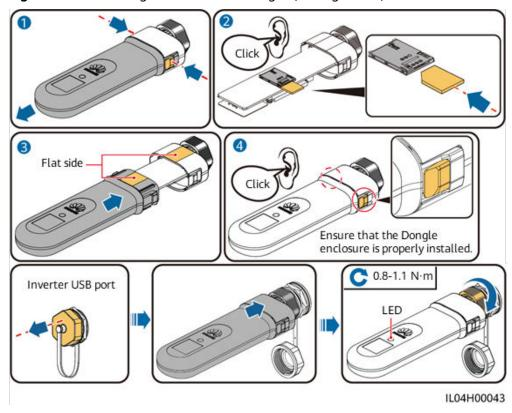
Figure 5-15 Installing the 4G Smart Dongle (SDongleB-06)
