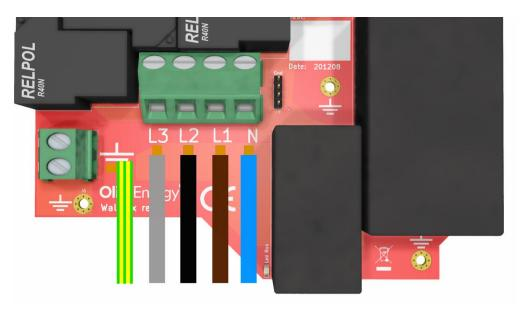
Fig. 9: Connection of lead-in conductor
