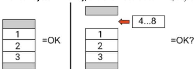
3. **If not okay**: The faulty module is probably one of the modules in the tower. Take one of the spare modules and exchange each of the remaining modules with the spare module one at a time. Check the battery status after each step. If battery status turns to "OK", the faulty module is the one that was exchanged.
